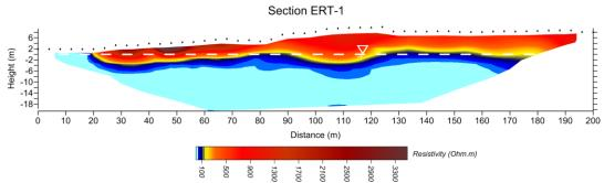
**Figure 6.** ERT -1 with topographic relief (5<sup>th</sup> iter., RMS 4.37%).
